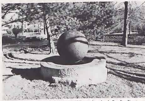
This pair of iron balls and granite troughs were used to grind gold at the Gray mine near Asheboro. Made in Belgium, they were shipped to Wilmington in the 1840s, were barged up the Cape Fear River to Fayetteville and were brought to Randolph County by wagon. Presently located on Marmaduke Circle, behind the home of J. D. Ross, Jr.
