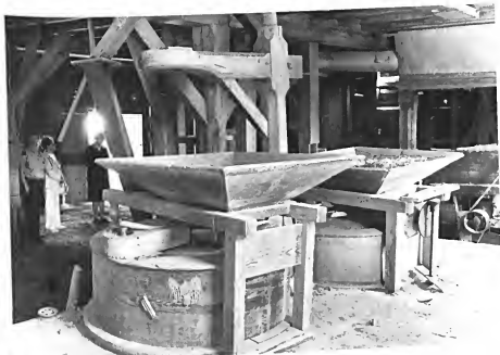
Interior of Miller's Mill, Trinity Township, showing the hoppers and housings of the wheat and corn stones (courtesy of Jane L. Delisle).
